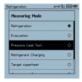
For the temperature-compensated leak test, a connection is established with available Bluetooth® probes. If cable probes are connected to the instrument, they are prioritized for the compensation.
