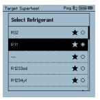
9.2 Setting the refrigerant: Press [▲] or [▼] to select the refrigerant and press [Menu/Enter] to confirm.
