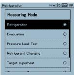
3 Press [▲] / [▼] to select Pressure Leak Test and press [Menu/Enter] to confirm.
