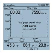
7 Start measurement: Press the [▼] (Start) key.
