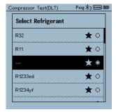
6.2 Setting the refrigerant: Press [▲] or [▼] to select the refrigerant and press [Menu/Enter] to confirm.
